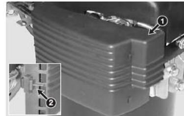
2. To the LEFT of the air filter there is a vertical metal lever running up the side of the engine (it can be felt if you put your hand against the engine block and slide it towards the back of the mower along the side of the engine).
